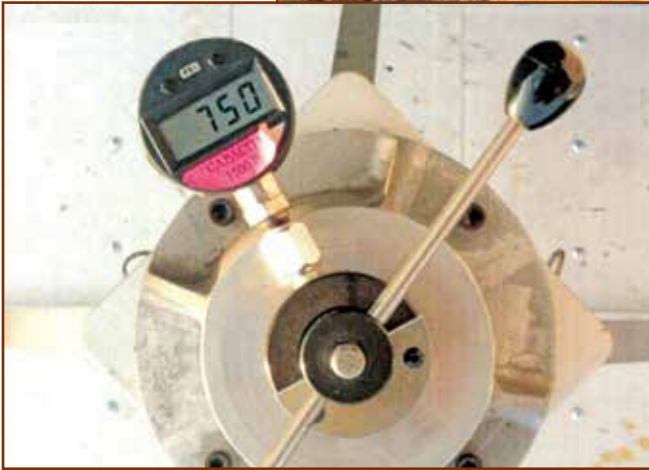
Photo 7 – Test result under field conditions yields pull test values in excess of 180 lbs. per square foot.
