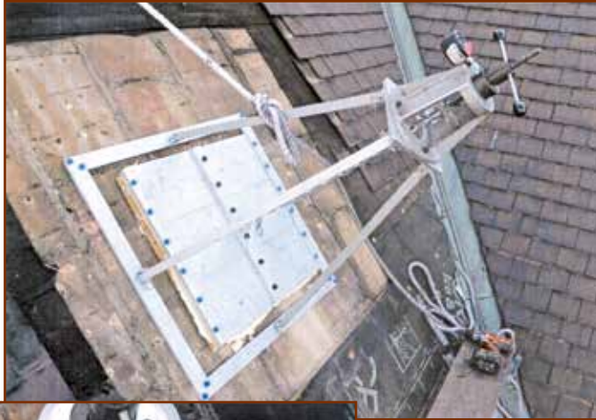
Photo 4 – Test apparatus set up for the pull test of the 2-ft. square panel fixed to the deck with low-rise foam adhesive under controlled conditions.
