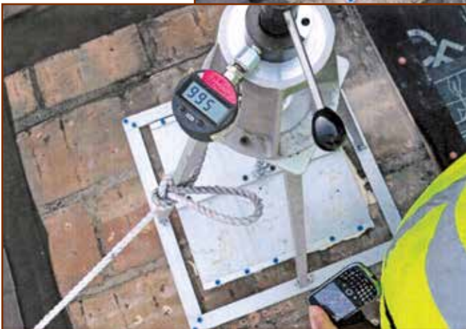
Photo 5 – Pull test values in excess of 140 lbs. per square foot derived under controlled conditions.
