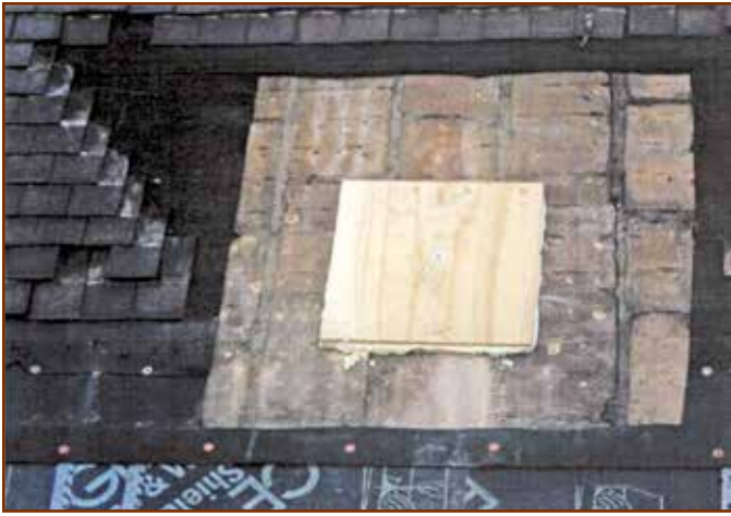
Photo 3 – Initial test panel set in adhesive to structural clay tile substrate under controlled conditions.
