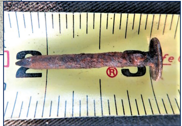
Figure 3. Corrosion of roofing nails observed at exploratory opening shown in Figure 2 . When wet for extended periods, wood-fiber products can be aggressive to some fastener types. Image courtesy of William J. Hope.
