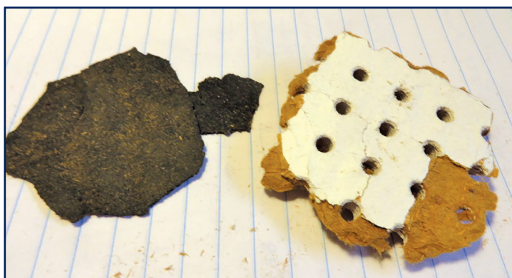
Figure 4. Samples of deck planks showing perforated underside which had been painted. The perforations impart appealing acoustic properties just as with ceiling tiles having equivalent design. Image courtesy of William J. Hope.
