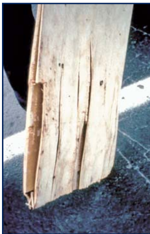
Figure 13 – Some first-generation FRT products experienced degradation from elevated attic temperature and humidity.
