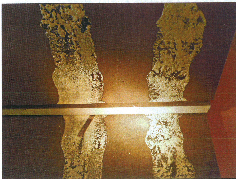
Photo 4 – Field mock-up sample assembled with known deflection (a shim was placed parallel to an edge condition of the lower board). The top board was “walked in” as recommended by most manufacturers. The temporary load distributed the adhesive horizontally across both the upper and lower boards, yet no bond was achieved.
