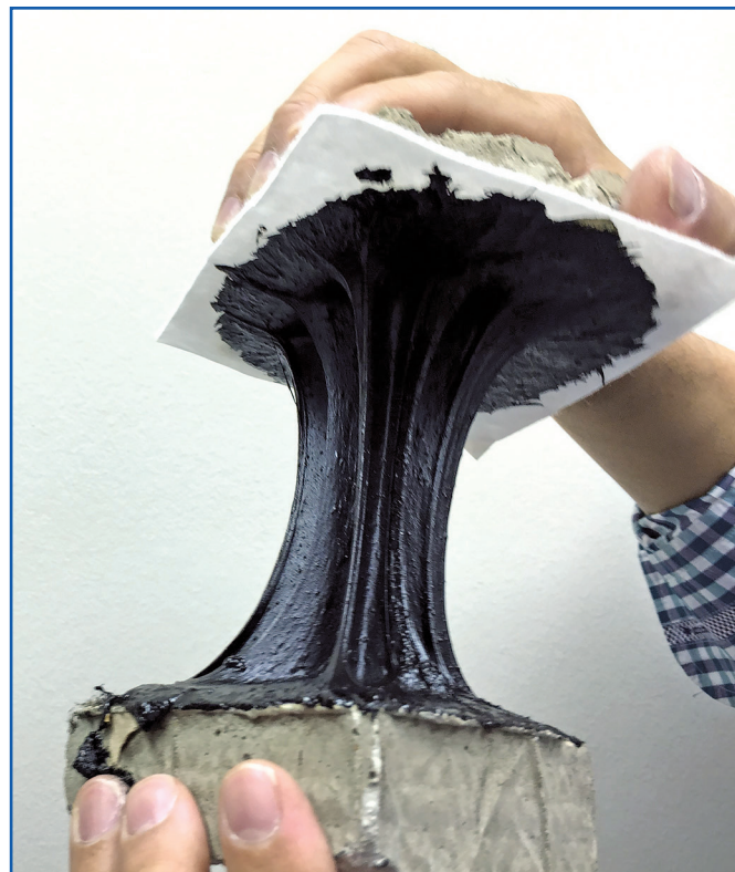
Figure 5. This photo demonstrates the high elasticity of polymer gel.
