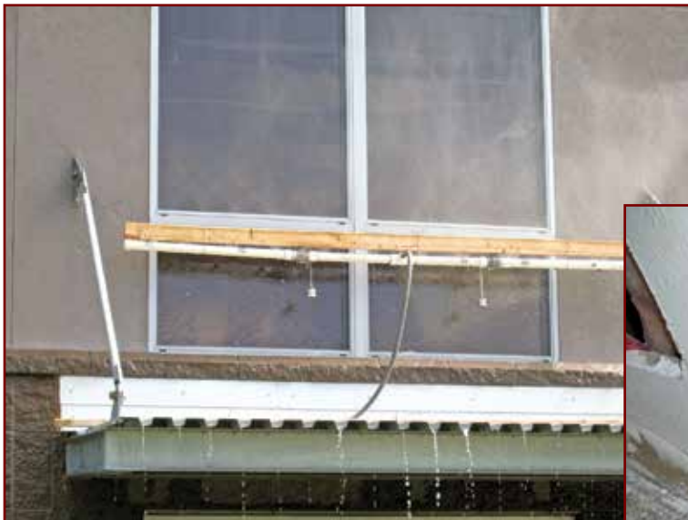
Photo 1 – Spray-bar water testing.
