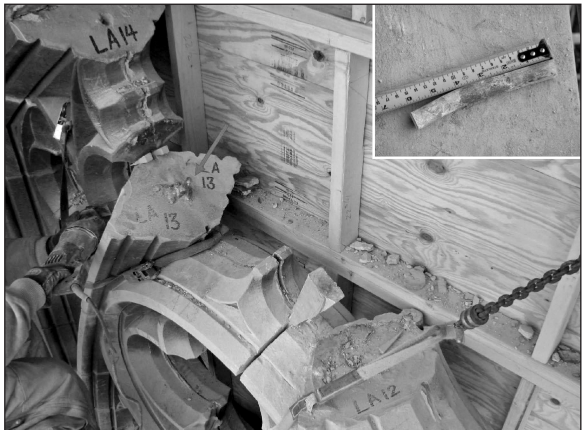
Photo 17 – Overall condition of steel pins at stone cusps from the organ loft window location.
