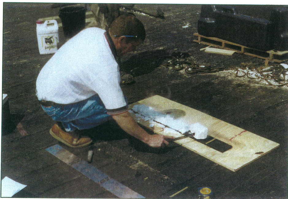
Photo 8: Covering the removed sample with a blanket of dry ice prior to separating the felts.
