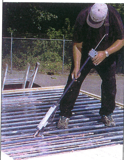
Photo 8: Covering the removed sample with a blanket of dry ice prior to separating the felts.
