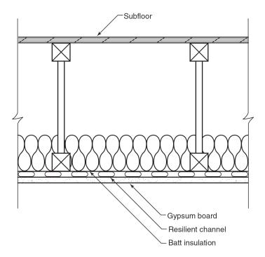
FIGURE A.8.15.1.2.6 Combustible Concealed Space Cross Section.
